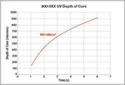
The product was UV cured using an F300S/F300SQ Fusion UV System equipped with a standard "H" bulb.
